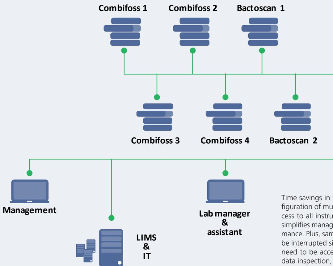
Time savings in the laboratory: with central configuration of multiple instruments and central access to all instrument data, the Mosaic software simplifies management of instruments and performance. Plus, sample throughput does not need to be interrupted since the instrument PC no longer need to be accessed for configuration changes, data inspection, data export etc.
