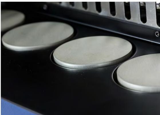
Hotplates with individual temperature control and automatic shutdown feature that allows out-of-hours operation.
