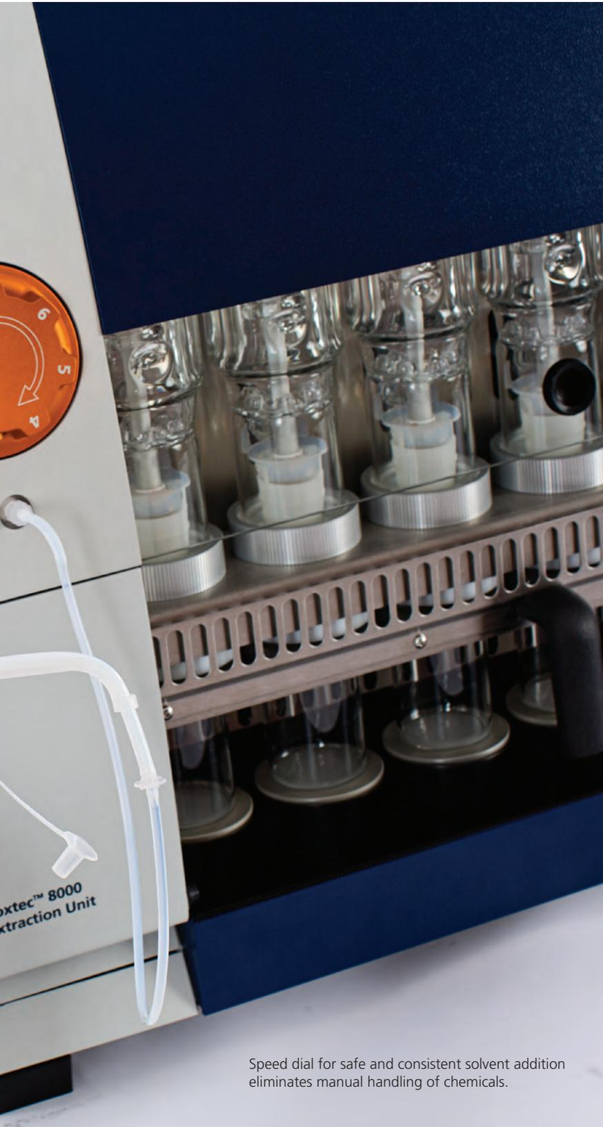
Speed dial for safe and consistent solvent addition eliminates manual handling of chemicals.
