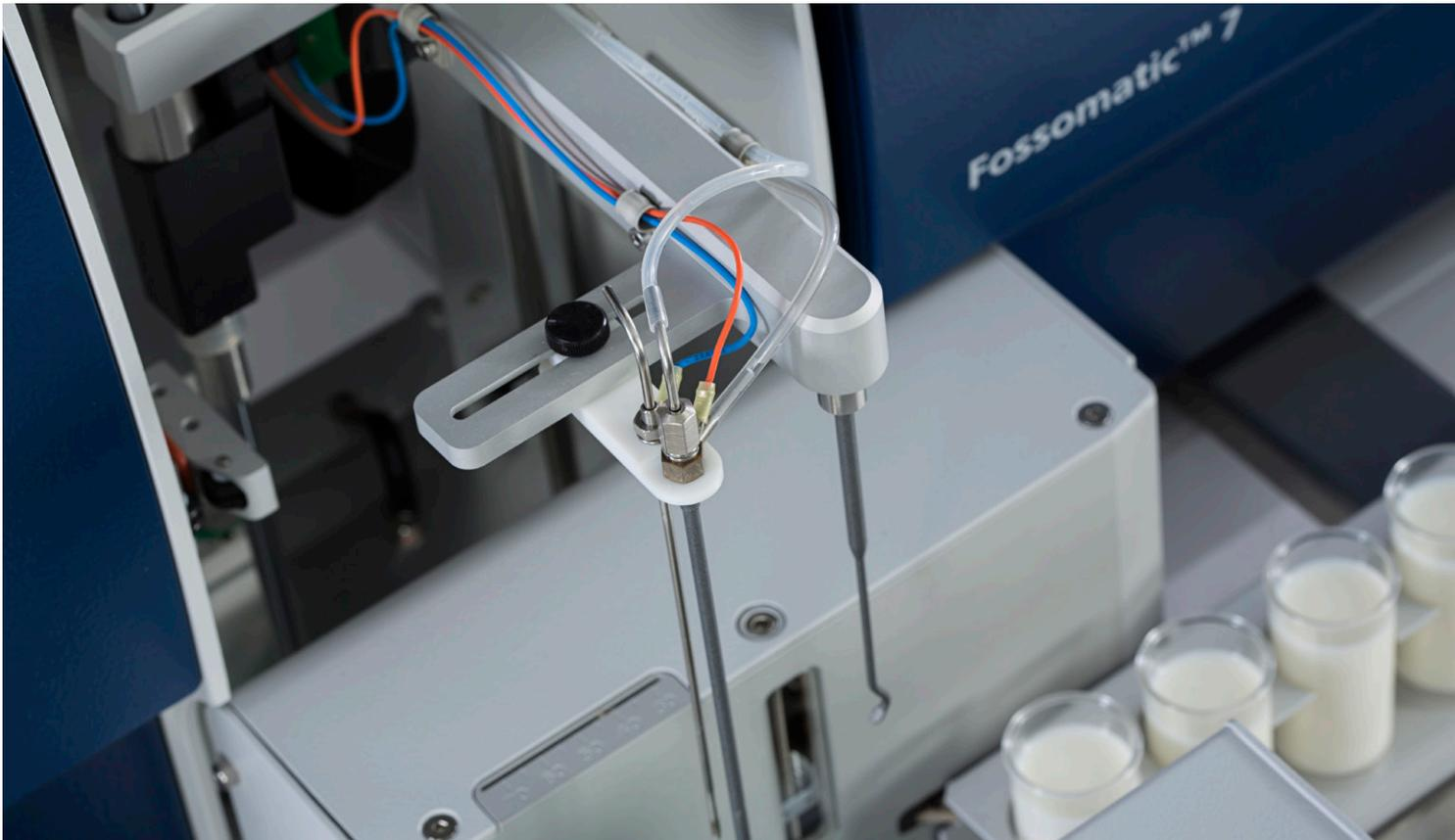
The Fossomatic™ 7 and Fossomatic™ 7 DC provide accurate somatic cell counting and differential somatic cell counting capability (Fossomatic 7 DC). Both models handle up to 600 samples per hour and are based on flow cytometry technology that counts somatic cells in compliance with ISO/IDF and FDA/NCIMS standards. Results are delivered simultaneously in six seconds while unique hardware and software features boost proficiency in the laboratory.
